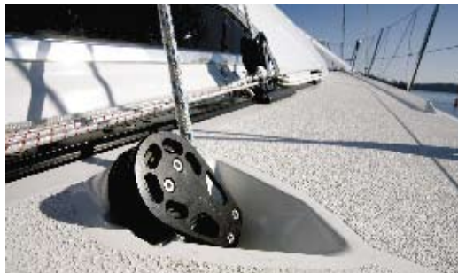
X-Yachts' mainsheet system and genoa car adjustment led back to the cockpit.
