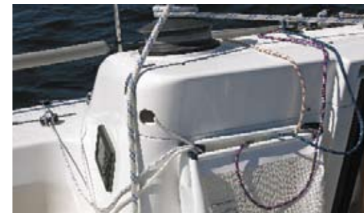
Genoa inhauler line adjusted from the cockpit.
